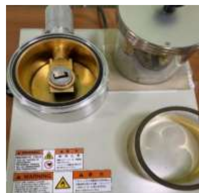
FIGURE 2. JEOL vacuum coating device
