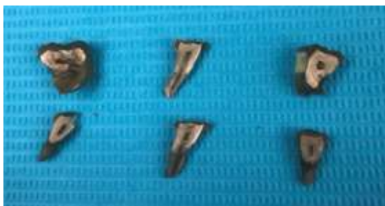
FIGURE 3. Experimental samples coated with a 10 nm thick layer of platinum
